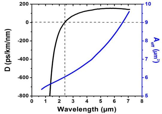
Fig. 2. Numerical modeling of the fundamental mode of the suspended-core chalcogenide fiber, showing the chromatic dispersion curve (upper, black curve) and effective mode area (lower, blue curve).
