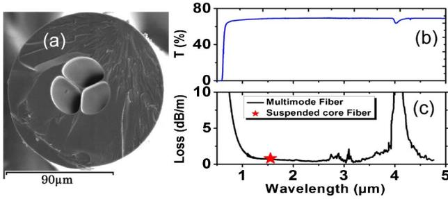
Fig. 1. (a) Profile of the chalcogenide  $\text{As}_2\text{S}_3$  suspended-core fiber captured by means of scanning electronic microscopy, (b) chalcogenide bulk transmission, and (c) optical loss of the mono-index large core multimode fiber as a function of wavelength. Loss measured at  $1.55 \mu\text{m}$  for the suspended core MOF (star).
