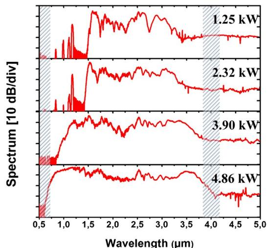
Fig. 4. Experimental recording of SC generation in a 20-mm-long sample of suspended-core chalcogenide fiber for pump peak power increasing from 1.25 to 4.86 kW. The main features of the  $\text{As}_2\text{S}_3$  transmission window are also displayed by means of hashed areas, the glass band gap (hashed zone at 0.6  $\mu\text{m}$ ) and SH absorption band (hashed zone at 4.0  $\mu\text{m}$ ).
