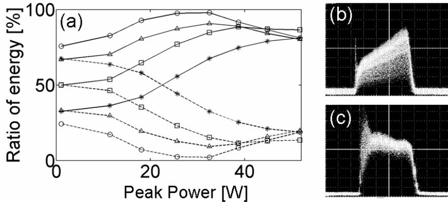
Fig. 3. (a). Experimental evolution of the energy ratio contained in the right (solid line) and in the left (dashed line) circular polarization as a function of the pump/signal power for four different initial signal polarization states. Output scrambled signal at  $P = 1$  W (b) and at  $P = 45$  W (c).
