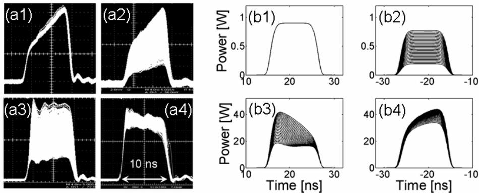
Fig. 4. Output pump (a1) and signal (a2) for  $P = 1$  W after scrambling of the input signal polarization. Output pump (a3) and signal (a4) for  $P = 45$  W after scrambling of the input signal polarization. (b1), (b2), (b3) and (b4) are numerical simulations corresponding Figs. (a1), (a2), (a3) and (a4), respectively.
