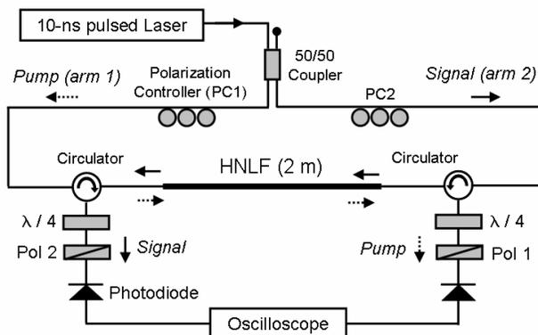
Fig. 1. Experimental set-up. HNLF : Highly Nonlinear Fiber,  $\lambda/4$  : quarterwave-plate, Pol : Polarizer.
