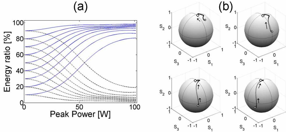
Fig. 2. Simulation results: (a) Evolution of the energy ratio contained in the right circular polarization (solid line) and in the left (dashed line) circular polarization as a function of the pump/signal power for different initial signal polarizations. (b) Evolution of the signal polarization state on the Poincaré sphere for four different input signal polarization states. The counter-propagating pump wave is injected with a right circular polarization ( $S_2 = 1$ ).
