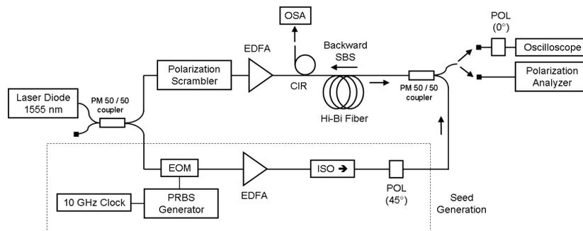
Fig. 3. Experimental set-up. CIR: Circulator, EDFA: Erbium-doped Fiber Amplifier, EOM: Electro-optic modulator, POL: Polarizer, ISO: Optical isolator, PRBS: Pseudo-random bit sequence, OSA: Optical Spectrum Analyzer.
