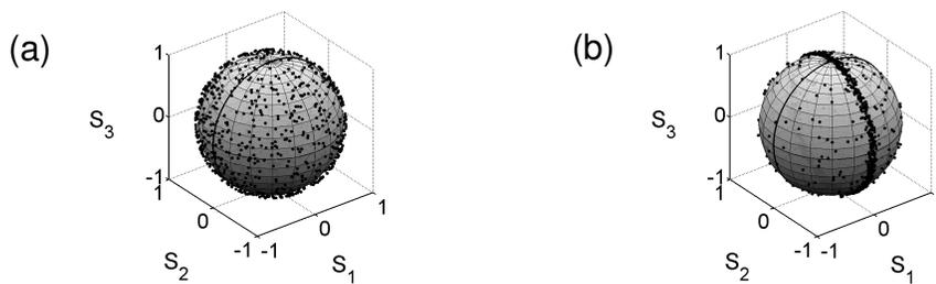
Fig. 5. Output polarization of the scrambled signal after propagation in the 200-m long PM-PCF for an input average power of (a) 100 mW and (b) 1100 mW.
