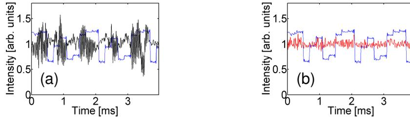
Fig. 7. (a) Output intensity profile of the scrambled signal propagating into the 500-m long PM-HNLF and passing through a polarizer, for an input average power of 10 mW (blue line) and 400 mW (black line) (b) same as (a) but in presence of a counter-propagating seed-signal.
