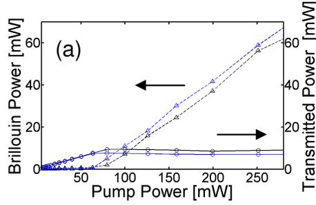
Fig. 1. (a) Experimental transmitted (triangles) and back-scattered Brillouin (circles) powers as a function of the input power for the fast (blue lines) and slow (black lines) axes of the 500-m long Hi-Bi fiber.
