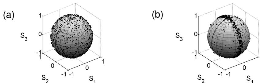
Fig. 4. Output polarization of the scrambled signal after propagation in the 500-m long PM-HNLF for an input average power of (a) 10 mW and (b) 400 mW.
