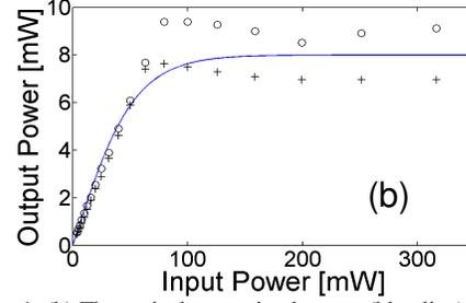
Fig. 1. (b) Theoretical transmitted power (blue line) as a function of the input power compared to the experimental data (circles and crosses).
