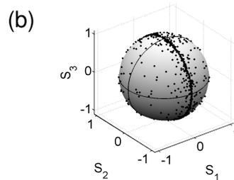
Fig. 2(b). Polarization of the output signal plotted on the Poincaré sphere.
