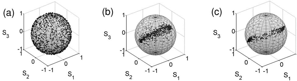
Fig. 6. Polarization of the back-scattered signal generated into the 500-m long PM-HNLF for an input average power of (a) 10 mW and (b) 150 mW (c) Same as (b) but for the 200-m long PCF and an input average power of 250 mW.
