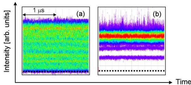
Fig. 8. (a) Intensity profile of the scrambled signal propagating into the 200-m long PM-PCF in presence of a counter-propagating seed-signal and recorded after the polarizer (a) for an input average power of 10 mW (b) 400 mW.
