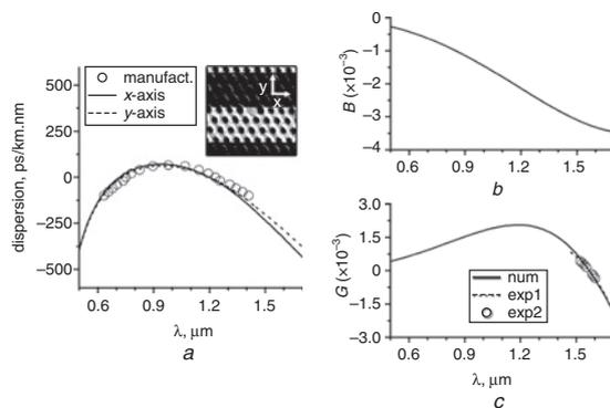
**Fig. 3** Numerical dispersion calculations of both fundamental orthogonal polarised modes of HiBi-PCF performed from SEM image of fibre cross-section (inset) compared to manufacturer data, numerical calculation of phase modal birefringence  $B$ , and numerical calculation of group modal birefringence  $G$  compared to experimental results obtained in telecommunication window
