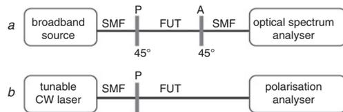
**Fig. 1** Experimental setups based on interferometric and polarimetric methods for group modal birefringence measurements
