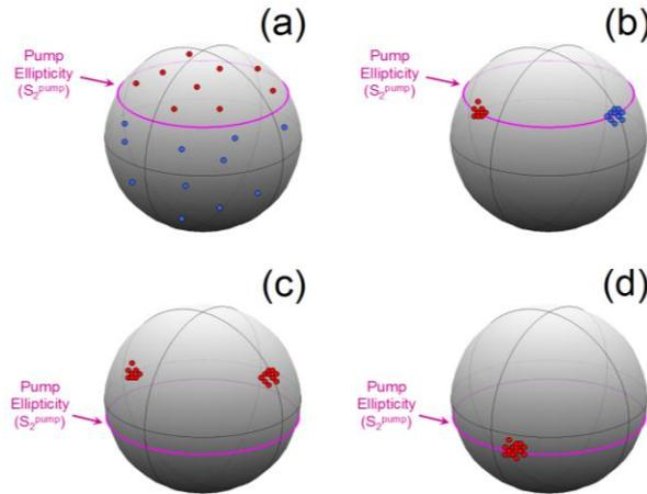
Fig. 1. (a) State of polarization at the input of a first isotropic section of fibre (b) Output of the first section (c) Input of the following section with change of the pump polarization (d) output of the section.
