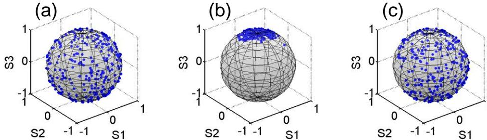
Fig. 3. Experimental observation of the polarization stabilization effect on the Poincaré sphere: (a) polarization of the signal wave at the system input (b) Signal polarization after nonlinear interaction with the counter-propagating pump wave. The pump and signal powers were 600 mW and 300 mW, respectively (c) Output polarization of the pump wave.
