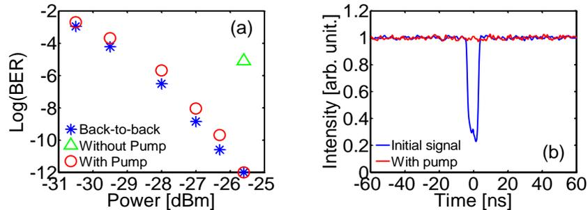
Fig. 5. (a) Evolution of the bit error rate as a function of average power in back-to-back configuration (blue crosses); at the output of the system, with polarization scrambling and after a polarizer with (red circles) and without (green triangle) the counter-propagating pump beam (b) Intensity profile of the 6-ns polarization burst observed after a polarizer by means of a low bandwidth oscilloscope, without (blue line) and with (red line) counter-propagating pump wave.
