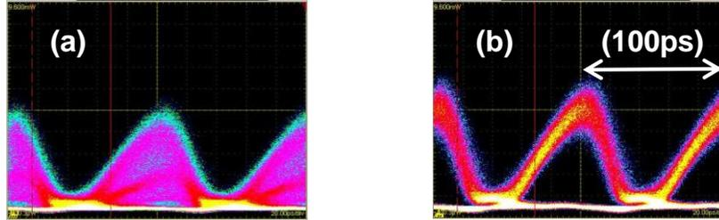
Fig. 4. Eye-diagrams of the 10-Gbit/s signal at the system output and monitored behind a polarizer (a) without and (b) in presence of the counter-propagating pump beam.
