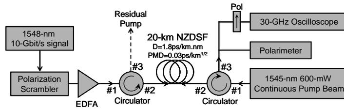
Fig. 2. Experimental setup. Pol Polarizer.
