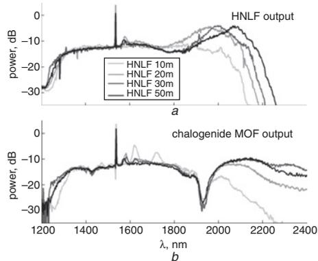
**Fig. 3** Generation of soliton gas at output of HNLF against fibre length, and corresponding supercontinuum extension after soliton gas injection into 50 cm-long chalcogenide MOF against initial HNLF length
