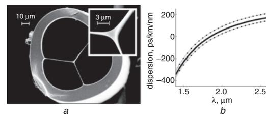
Fig. 2 SEM image of cross-section of chalcogenide microstructured fibre and (inset) magnification of suspended core, and MOF dispersion curves calculated from microstructure parameters obtained from SEM picture with  $\pm 10\%$  accuracy on fibre core size
