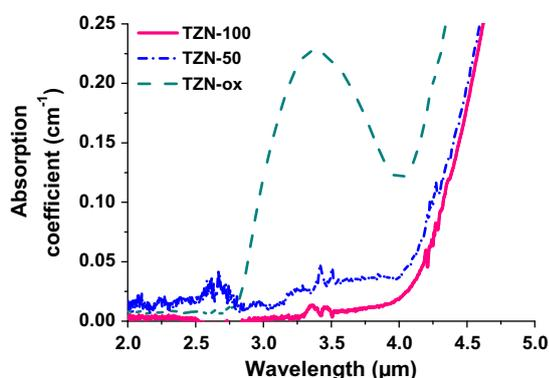
Fig. 2. TZN glasses absorption coefficients in the mid-IR range.
