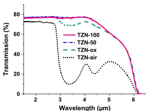
Fig. 1. TZN glasses IR transmission spectra for 4 mm thick slices.
