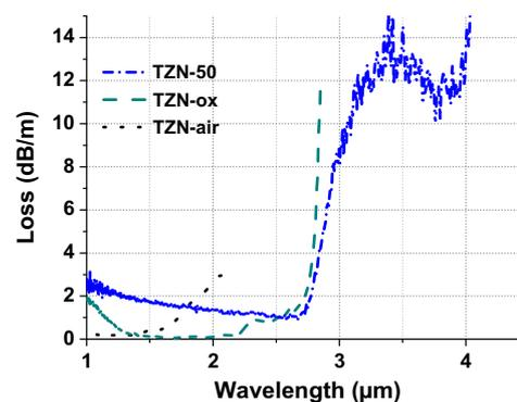
Fig. 3. Spectral losses of fabricated single index tellurite fibers.
