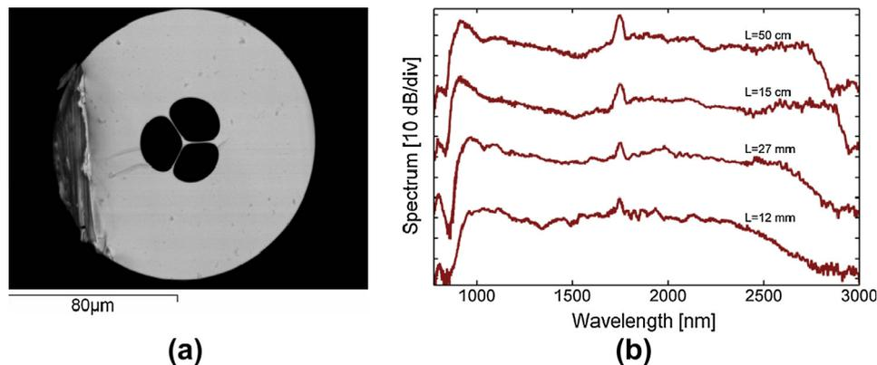
Fig. 4. (a) SEM picture of the TZN-50 MOF cross section, (b) supercontinuum generation recorded for various lengths of our TZN-50 tellurite suspended core fiber.
